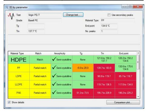
The table above illustrates how the plastic has been correctly and unambiguously identified as HDPE, based upon matching the parameters stored within the **identiPolQA** memory.
